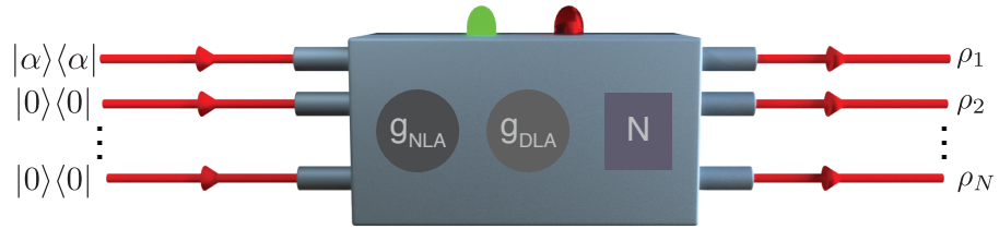
Figure 8.4: Hybrid Cloning Machine. An N -port hybrid cloning machine (HCM), consisting of two control knobs: a probabilistic noiseless linear amplifier (NLA) gain ( g_{\text{NLA}} ) and a deterministic linear amplifier (DLA) gain ( g_{\text{DLA}} ). Heralded successful events (symbolised by a green light) produce N clones ( \rho_i ) of coherent state |\alpha\rangle with noise less than the deterministic approach, while unsuccessful events (red light) will be discarded.
