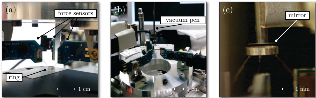
Figure 9.3: Different steps in the preparation of the stage for the upper mirror. (a) Attaching the supporting ring to the tips of the three force sensors. (b) Holding the mirror with the vacuum pick-up pen during positioning. (c) Close-up of the mirror held by the vacuum pick-up pen just before releasing it onto the ring.
