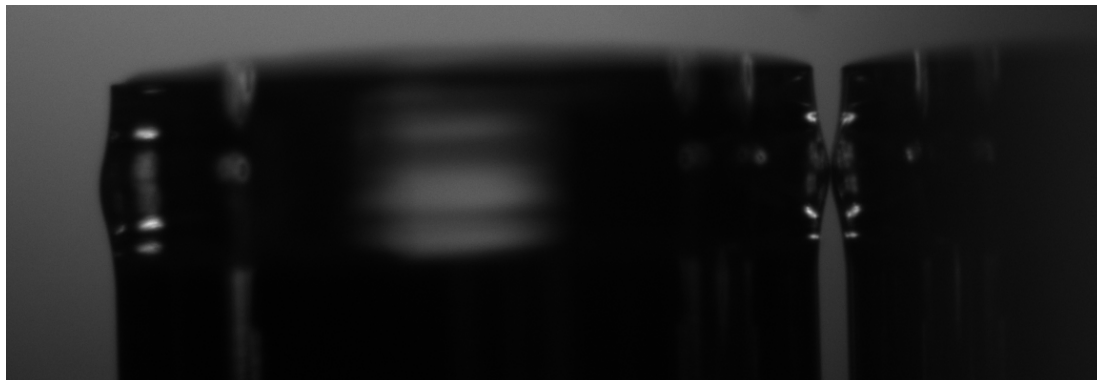
Figure 15.2: Prism coupling the smallest of the resonators that we produced, a \text{LiNbO}_3 whispering gallery resonator with a 1.4 mm diameter and 200\ \mu\text{m} polar radius. The reflection of the resonator (on the right of the image) can be seen in the prism.
