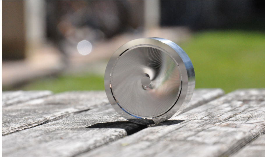
Figure D.3: Image of a charge 10,000 vortex mirror. The optic consists of 125 steps, each imparting a phase shift of 80 \times 2\pi .
