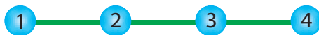
Figure 9.1: Four-mode linear cluster state. Resource state for demonstrations of one-way quantum computing; can be viewed as a blank quantum circuit board. Each numbered circle denotes a quantised optical mode (qumode), and the green links between them have edge weights of unity, as defined in the graphical calculus of reference [22], and treated in section 7.2.
