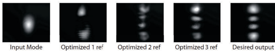
Figure 5.11: Progression of conversion from a TEM_{00} mode to a TEM_{30} mode. The CCD images after each reflection from the deformable mirror are shown. The final mode conversion resembles the desired output, but is not a perfect conversion. Source: [54].
