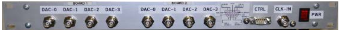
Figure 4.4: Digital Locking Racks. (a) ADC rack with: Clock - 80 MHz input; inputs - IP_{x.1} and IP_{x.2} ; and combined outputs OP_x that is then sent to a DIO terminal on the PXI chassis. (b) Clock rack with: CLK-IN - 80 MHz input; CTRL - FPGA control input; and DAC-x - frequency outputs.
