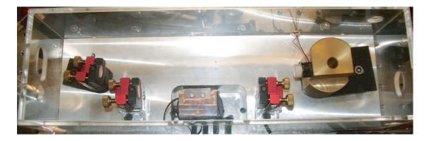
**Figure 3.3:** Photo the optical parametric oscillator. The crystal is pumped from the right from one of the curved mirrors. The infrared exited from the top left mirror. The ensemble was enclosed in a perspex box to minimize air currents.
